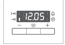
When the time has elapsed, the function indicator flashes, an audible signal sounds for 2 minutes and the oven switches itself off.
